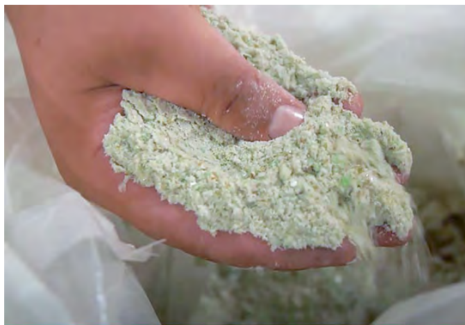
Figure 3.11 Glass Crushed to Sand (Courtesy Aqua Tools)
