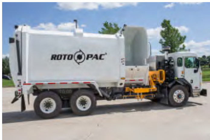
Figure 3.8 ROTO PAC Organic Waste Collection Truck with Auger Packing System
